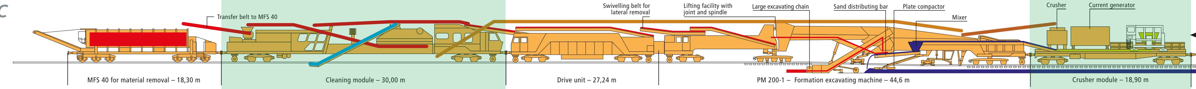
**PM 200-1 BR/C – a formation rehabilitation machine in modular design**
