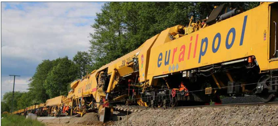
A formation rehabilitation machine in modular design. It can be optionally used to completely renew ballast, clean ballast or produce grade 2 mixture from existing, old ballast in combination with track-bound formation rehabilitation. It can be used in periods of possession of 7 hours and over.
