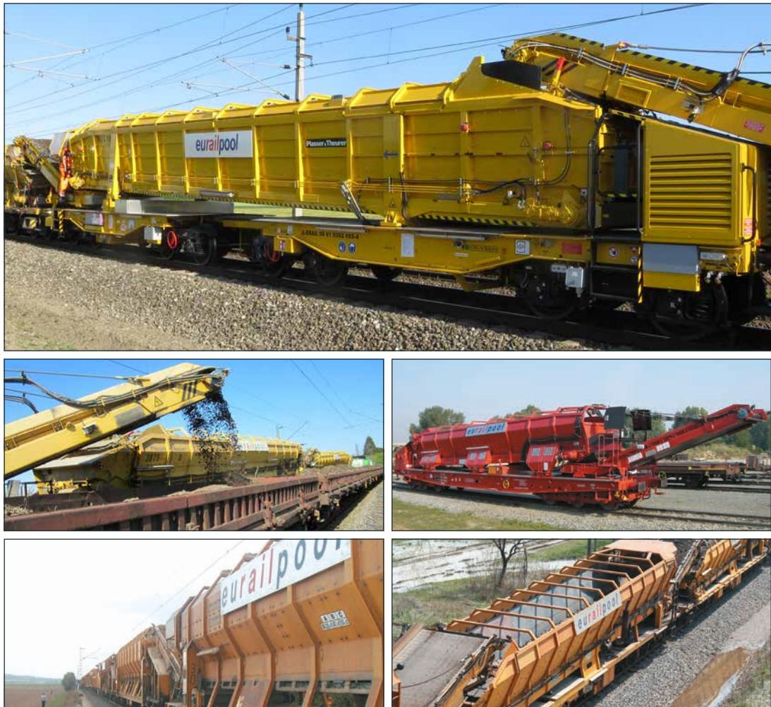
The material conveyor and hopper units serve both to supply material and to transport the excavated material away without using the adjacent track. Loading is carried out using a wheel loader or excavator via a loading station or directly into the MFS. The excavated material is unloaded to temporary storage sites or onto K wagons via swivelling conveyor belts.
