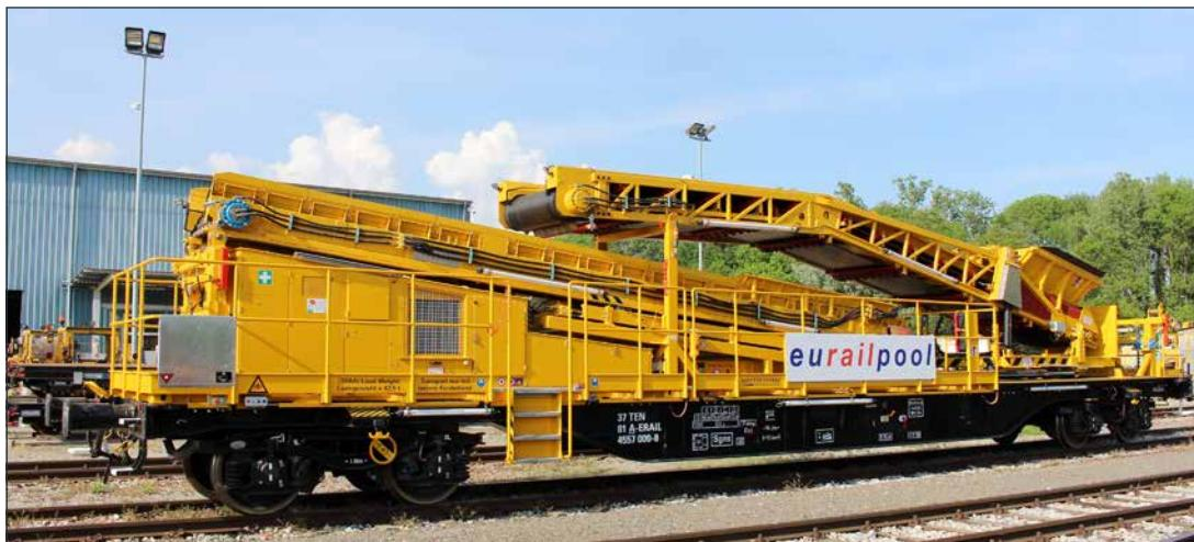
The VLA serves to round off the product range. It is used to dig up the edge paths in front of a formation rehabilitation machine. If necessary, the loading belt is extended from the MFS. The transfer wagon serves to load the excavated material at a distance of up to 8.50 m away from the track axis.
