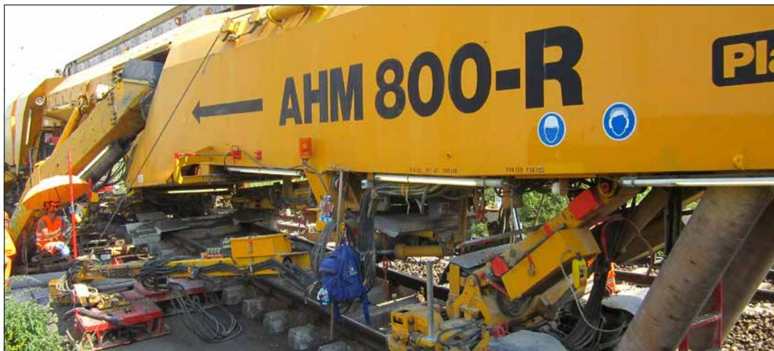
The AHM 800-R is used on sections in which grade 2 mixture is installed. It is able to remove the ballast with the ballast excavating chain, crush it on the machine, mix it with new material and re-install it as a formation layer/frost layer. Installation of the new ballast is carried out in a separate operation.
